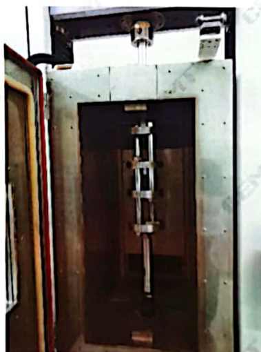
图5 垂直层向压缩强度试验及曲线 Fig.5 Compressive strength perpendicular to laminations test and curve
