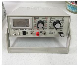
High insulation resistance measuring instrument
