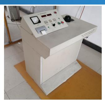
HT-100 Breakdown Voltage Tester
