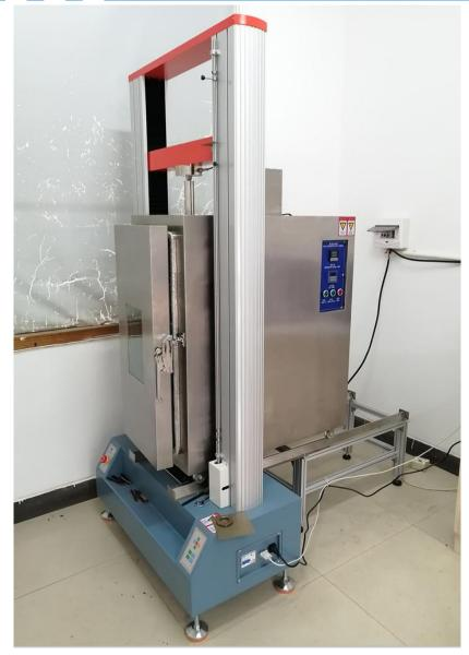
High temperature tensile testing machine
