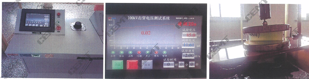
图5 平行层向击穿电压试验 Fig.5 Breakdown voltage parallel to laminations test
