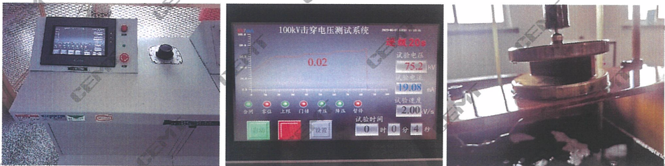
图5 平行层向击穿电压试验 Fig.5 Breakdown voltage parallel to laminations test
