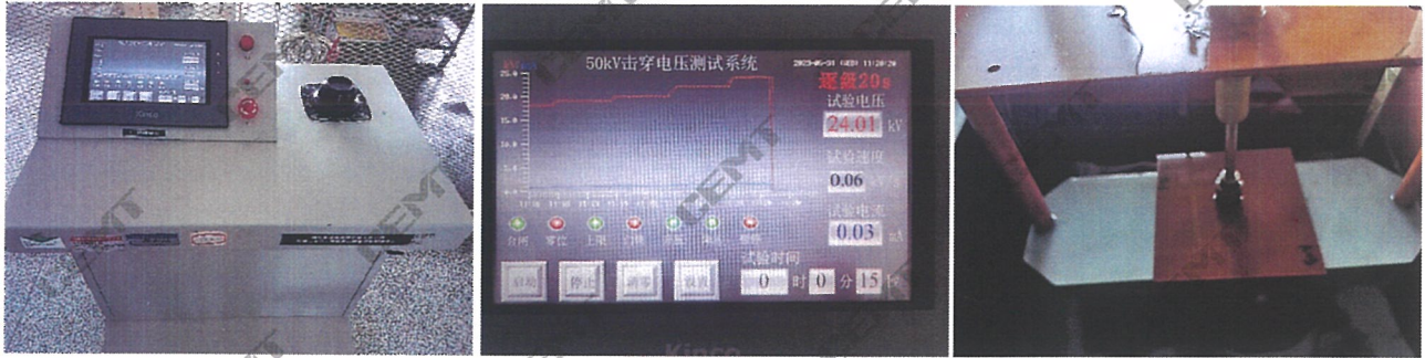
图4 垂直层向电气强度试验 Fig.4 Electric strength perpendicular to laminations test
